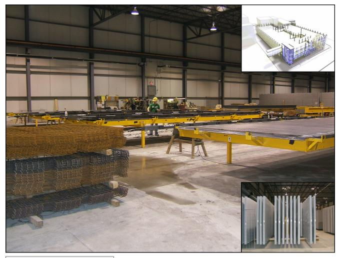
Project: CANADACAR System Guelph, Ontario <u>Owner:</u> Newton Parking Structures Ltd. <u>Precaster</u> Newton Parking Structures Ltd. <u>Product:</u> Each HPC precast panel is 9.00m long and joined together to produce the typical 18.00m module. Precast panel production floor at Newton Parking Structures Ltd. in Guelph, Ontario
