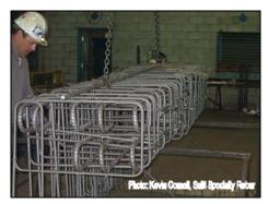
Stainless steel assembly wired into proper configuration at StelCrete.
