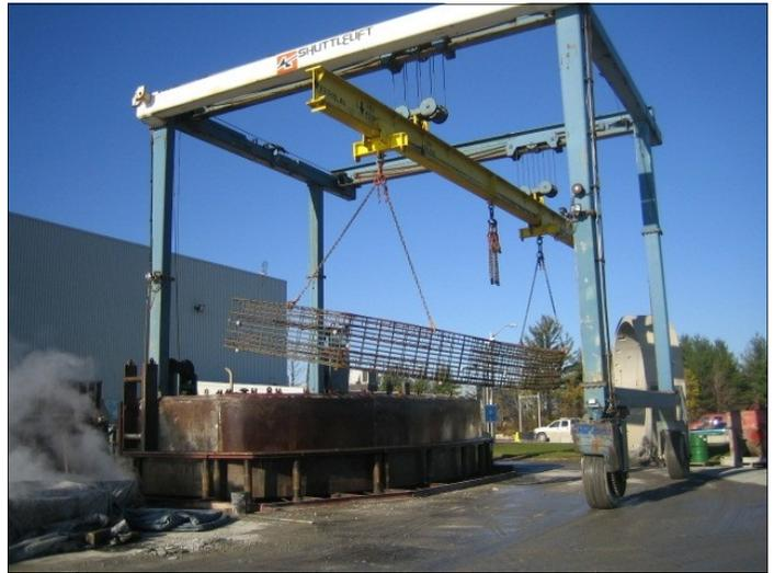
Mobile crane places cage into mold
